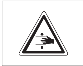
Risk of crushing
