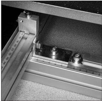
Loosen bolt to fix fence location needed for drilling.
